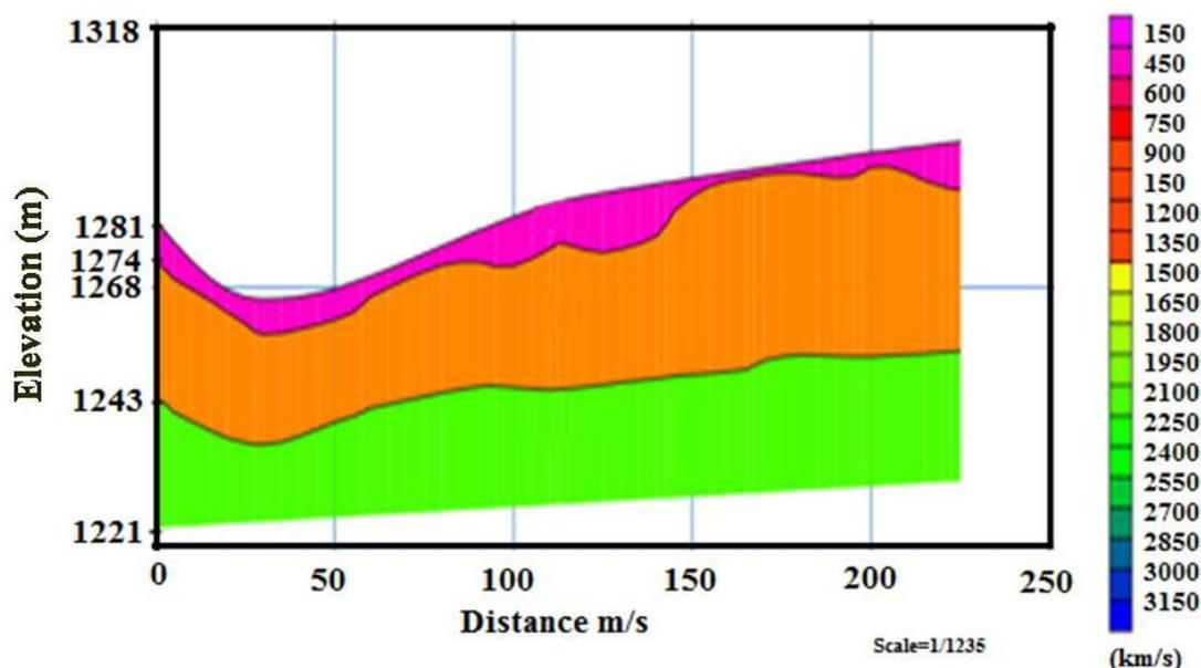
**Fig. 5** Tomographic section of subsurface lithology
