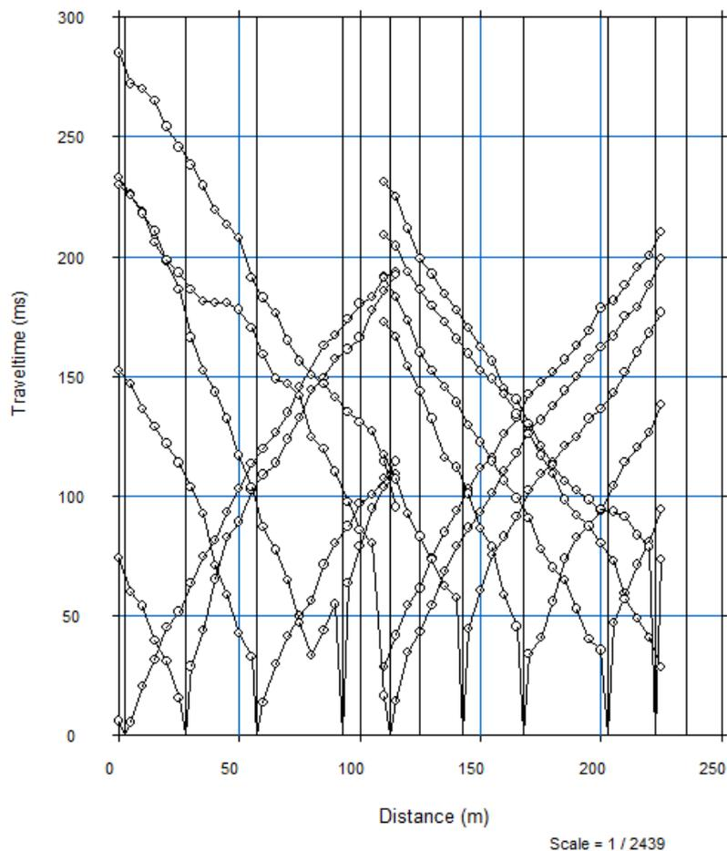
Fig. 4 The picked inversion of travel time curves for integrated profiles.
